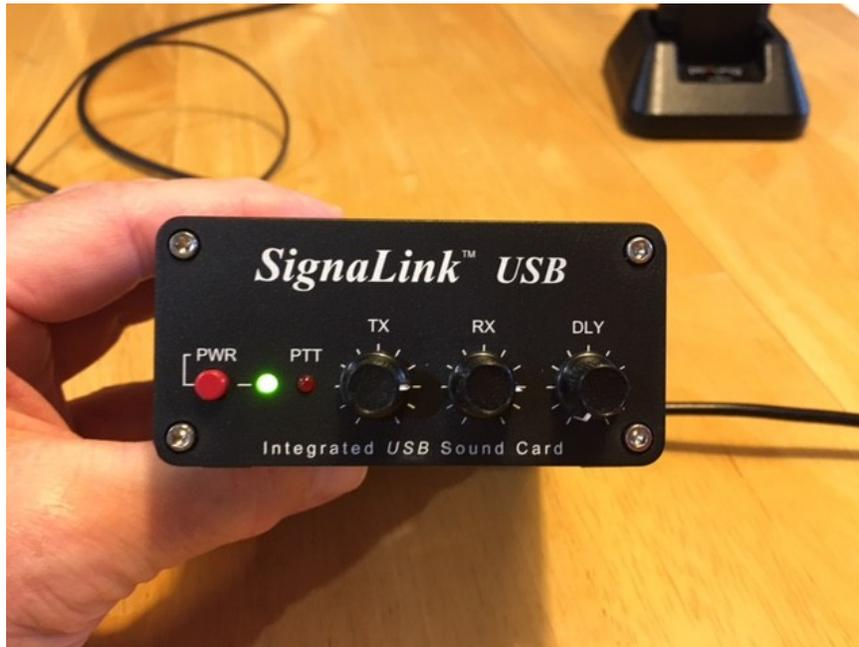
The above picture shows the Signalink settings I use for Packet WinLink QSO. Both the TX and RX are set at the 3 o'clock position, DLY is all the way counterclockwise.
