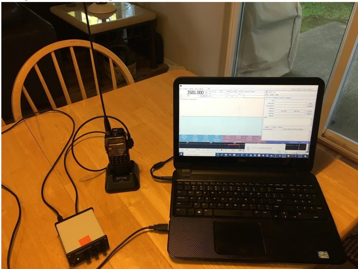
ordering process Tigertronics asked for type of ht. The Signalink→ computer usb cable and the Signalink→radio cable is included. Jumper wires and jumper wire instructions for your particular ht come with it. For an additional cost, Tigertronics offers a plugin IC board in lieu of the jumper cables. I have used both. The original jumper cables are still in use. However, I have broken the pins on 2 IC boards inserting them!
